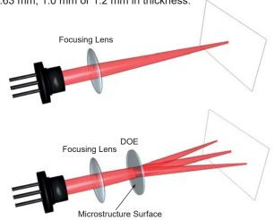
The DOEs are best used with collimated or slightly convergent laser sources (see figure to the left). The microstructure surface should be oriented towards the laser.
