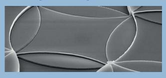
Direct write lithography processes are used to create either lithography masks or resist micro-relief profiles. Based on masks, micro-relief profiles are created by contact or projection lithography and subsequent etching processes like reactive ion etching to transfer the etch mask into the substrate.
