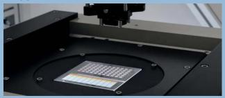
After fabrication, HOLOEYE will validate the compliance of the DOEs with the specification experimentally. For volume production of elements, optical key properties can be monitored using automated equipment.
