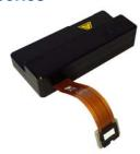
The LETO phase modulator is based on reflective LCOS microdisplays with 1920 x 1080 pixel resolution. With a pixel pitch of only 6.4  $\mu$ m and small interpixel gaps of 0.2  $\mu$ m the LETO SLM provides a high fill factor of 93% and
