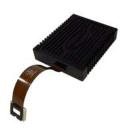
The GAEA-2 phase modulators are based on reflective LCOS microdisplays with 4160 x 2464 pixel resolution and 3.74 µm pixel pitch. The phase displays can be addressed at 3840x2160 pixel or 4000x2464 pixel
